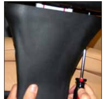
8. Slide new shroud up and into position for attachment.
