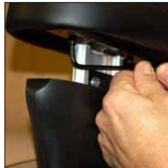
7. Securely attach the arm pad with the 3/16" Allen-heads bolts.
